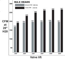
The 360 MA-X heads from Indy are true Magnum heads. The MA-X utilizes 100% Magnum style parts including pedestal mounted rockers, magnum bolt pattern intake manifolds and valve covers. The big advantage to the MA-X Head is the dual exhaust bolt pattern. Both stock Magnum as well as W-2 bolt patterns are machined into the head allowing for a much larger header selection
