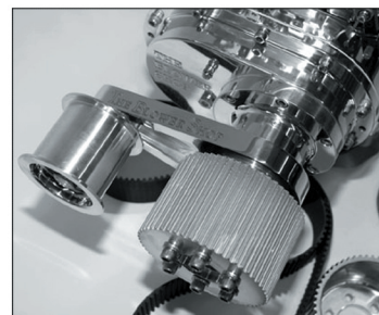
Belt adjustment 4" idler pulley bracket and stand shown
